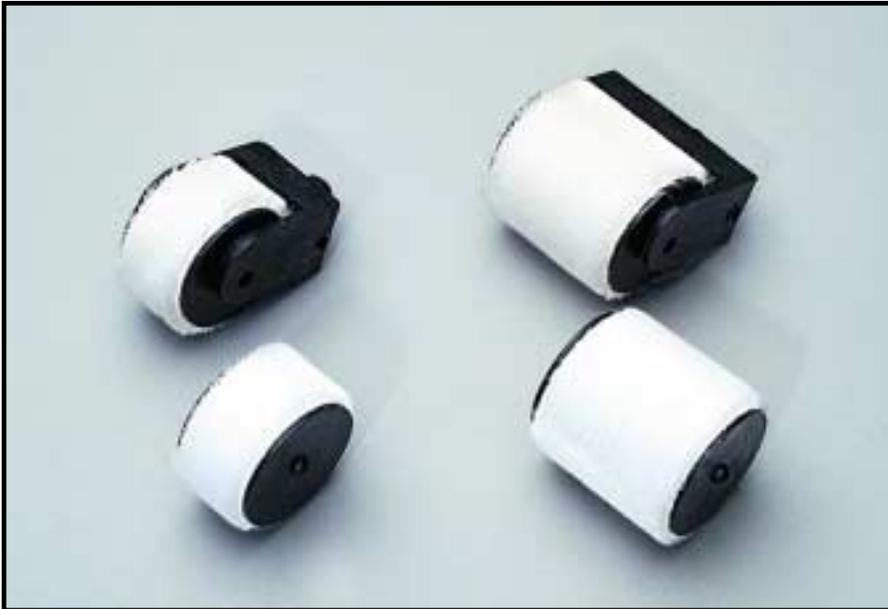
Semco® roller nozzles are designed to apply adhesives and sealants evenly over a wide area of substrate. They are ideal for the application of faying surface sealants. The 1/4 NPT male threaded end can be used with any of the Semco® line of disposable cartridges and Semkit® packages (i.e. 1, 2.5, 3.5, 6, 8, 12, 20, 32 oz. and 1/10 gallon sizes).
